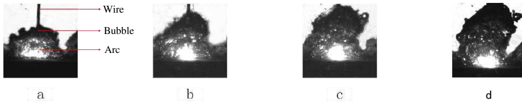
FIGURE 3. Underwater wet welding images
