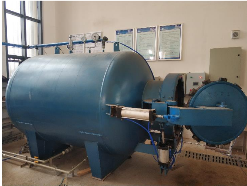
FIGURE 1. Underwater wet welding experimental system
