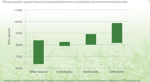
Energy content measured in British Thermal Units per pound of several potential biomass feedstocks. BTU per pound provides a relative measure of the amount of energy that can be released from a given feedstock in a combustion or thermocemical conversion process. Switchgrass falls within the range for woody feedstocks and is at the high end of the range for other perennial grass species.
